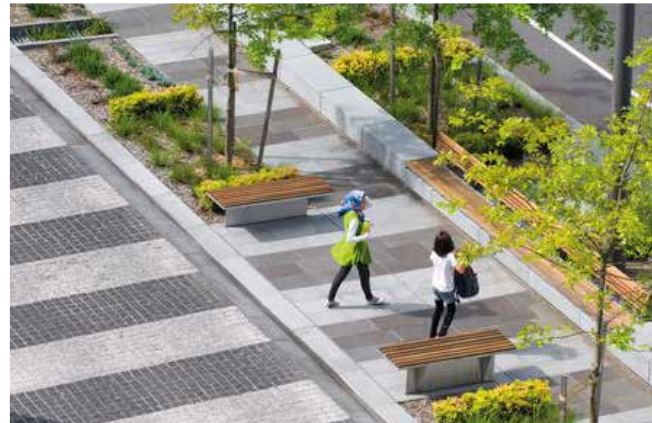
Paving used to delineate between pedestrian and vehicle zones
